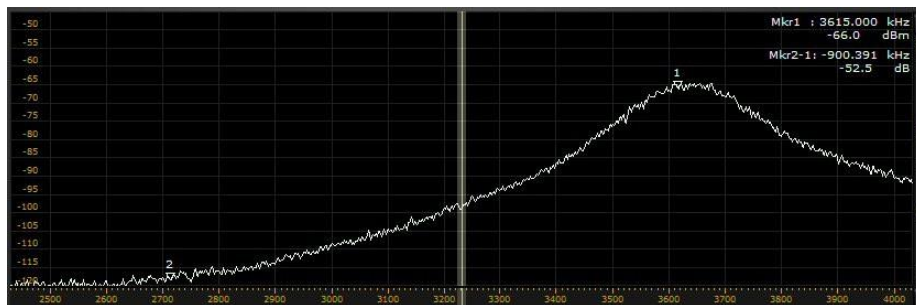
Figure 2.2 Actual plot of RF bandpass filter on 80m
