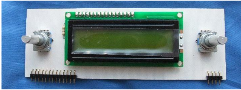
Figure 8.9 Completed Display PCB (Old PCB shown) New boards are commercially made
