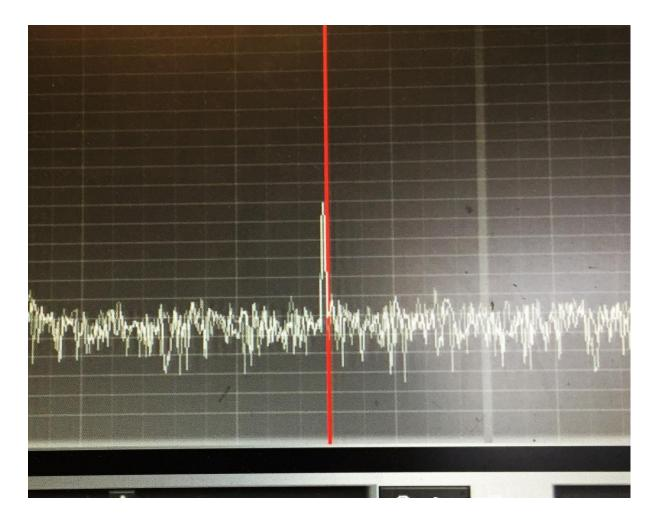
This one shows the carrier modulated with a 1kHz signal...
