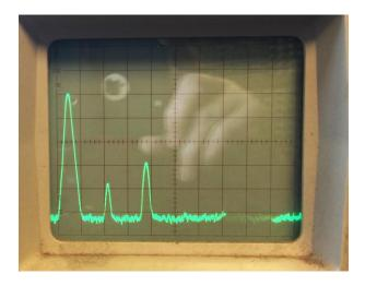
Using single ended PAs there are even as well as odd harmonics emitted and is the reason why push pull is used in this project along with providing more output from the same applied PA voltage. A Low Pass Filter (LPF) is fitted between the output of the PA and a resonant antenna for the band or the antenna via an ATU. The filter is constructed to cut off or greatly attenuate before the third harmonic as the second harmonic is normally very much attenuated with a push pull output
