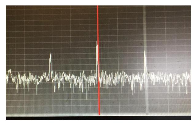
It can be seen that the carrier does not change in amplitude when modulation is applied. It is the sidebands (audio modulation) that changes in amplitude during different levels of audio. The receive station receiving a steady 'S9' on the signal meter with an un-modulated transmitted carrier will
